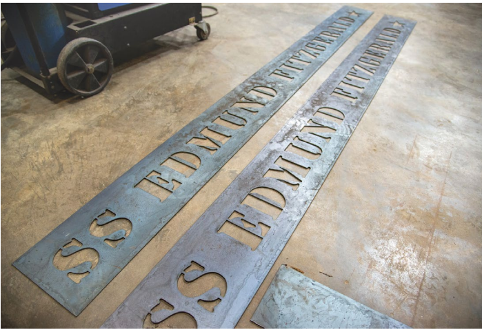
The name of the ship was cut out of two pieces of steel. Matt would later merge the two together and shape it into a hoop for the weathervane. When complete, the circumference was nearly 19 feet.
