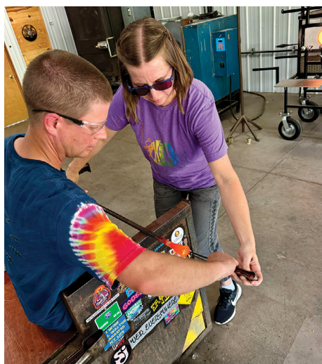
Glassblowing class teaching a student how to use steel tweezers to shape the inner swirl of a paperweight
