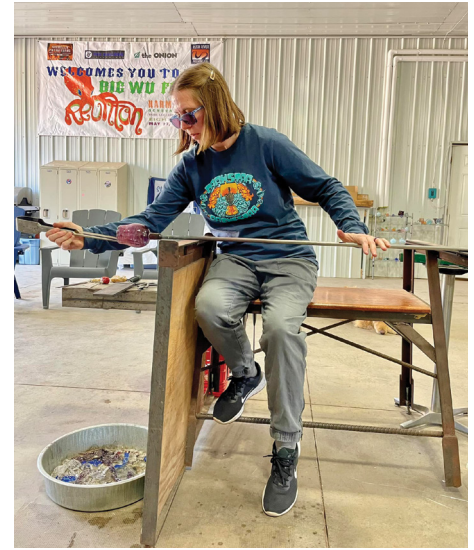
Using jacks to open up the mouth of a blown cup while on the glassblowing bench
