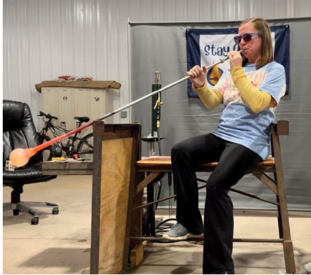
Blowing a bubble in the hot shop. The hot glass is clear, but appears yellow when hot. Gently blowing air through the hollow blow pipe inflates the glass.
