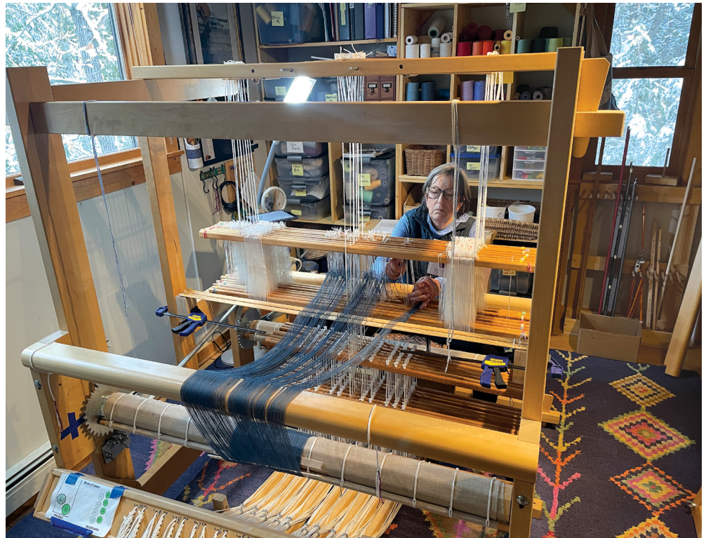
Toika Eeva loom being warped for small sample Overshot weaving project.
